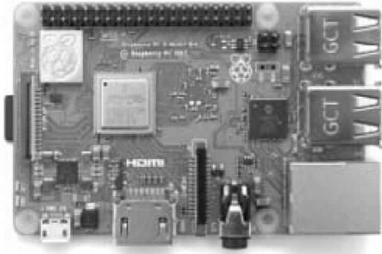
Abb. 11.11: Raspberry Pi 3, Model B+ (Quelle: Raspberry Pi Foundation)
