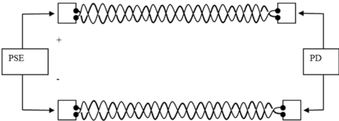
■ Abb. 14.41 Power over Ethernet IEEE 802.3af: Spare-Pair-Einspeisung
