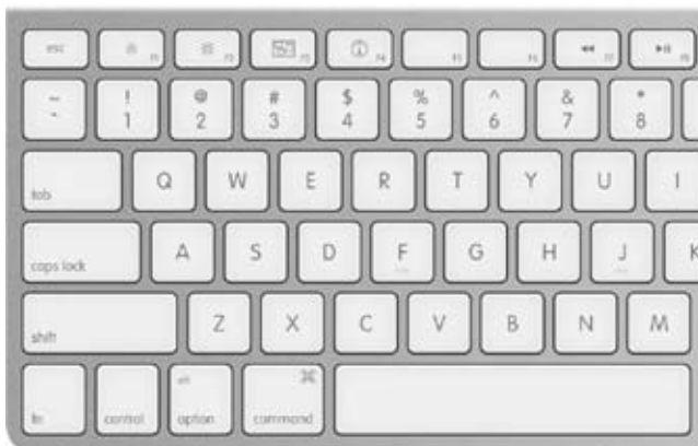
Figure 6-1: On the top row of aluminum Mac keyboards, the F-keys have dual functions. Ordinarily, tapping the F1 through F4 keys correspond to Screen Dimmer, Screen Brighter, Exposé, and Dashboard. Pressing the Fn key in the corner changes their personalities.
