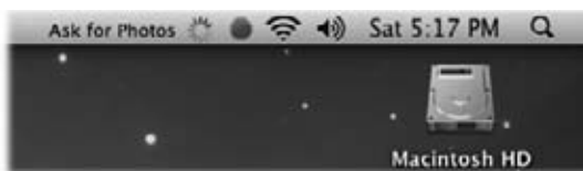
Figure 7-6: The three-part menu-bar indicator tells you that the workflow application is, in fact, running (the spinning progress indicator)—and, more specifically, which action is running (the text next to it). If you want to cancel a workflow halfway through, click the Stop sign.
