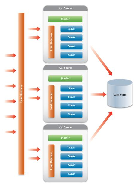
Internally to each server, the iCal Server spawns a number of slave processes equal to the number of processor cores, and the internal software load balancer distributes the connections across its slave processes. As each iCal Server reads from and writes to user calendars, it does so from the shared storage pool.
