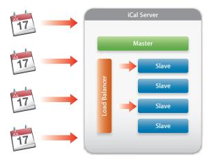
For these processes to be balanced, they must have a shared storage location. This can be as simple as a single file system location for a multiprocessor Xserve. If the processes are spread between several servers, the servers must use a shared storage solution like Xsan.
