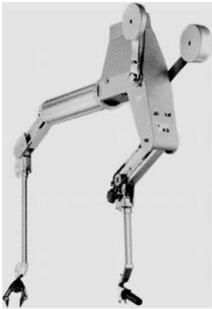
Abb. 8.2 Manipulator zur Handhabung radioaktiver Stoffe (Oxford Technologies) http://www.oxfordtechnologies.co.uk
